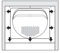
Screw the front panel to the machine door.
